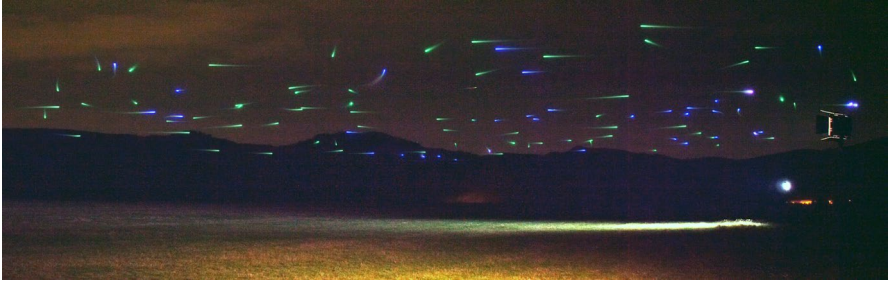
Fig. 6 Post-processed image of the raw video footage of the field experiment with 100 drones performing autonomous decentralized traffic in two layers. The image was created iteratively, by adaptively averaging consecutive video frames into a background image, and then getting the pixel-level lighter color values of the algorithm: green means free motion, blue means the drone is avoiding others, purple means the drone is queueing, white flash indicates that the target has been reached
