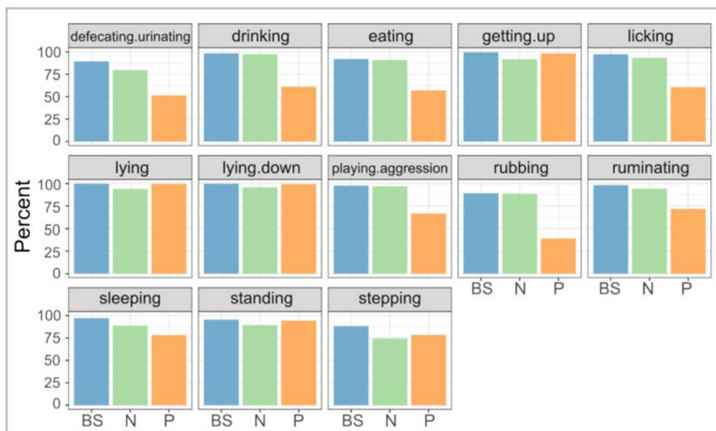
Fig. 13. F1 Score values of SVC classifier with different sensors: both sensors (BS), Noseband (N), and Pedometer (P) with settings Padding = 3; Window = 10 and Train size = Validation size = 0.5. Most movements were recognized better with Noseband than Pedometer.
