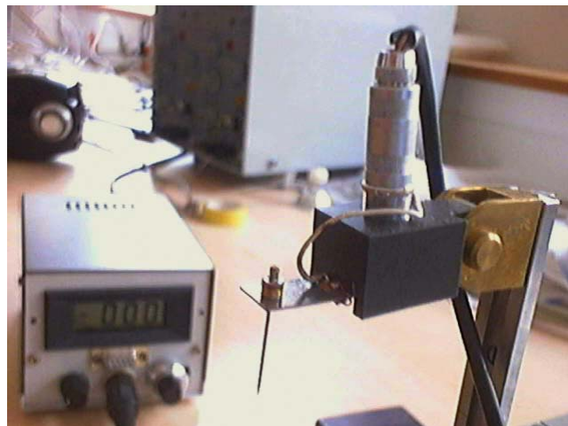
Figure 3.19. The third loading instrument with a built-in strain gauge and a digital display
