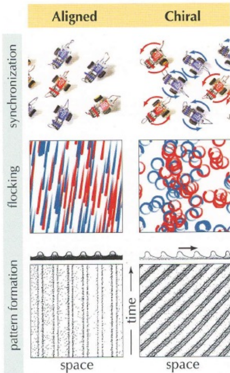
Figure 9.17. Nonreciprocal interactions between two species, R (Red) and B (Blue), induce a phase transition from static alignment to a chiral motion that spontaneously breaks parity. Top: nonreciprocal synchronization. Angular variables with nonreciprocal interactions drawn as robots spontaneously rotate either clockwise or counter-clockwise, despite no average natural frequency ( \omega_m = 0 in equation (9.63)). Middle row: non-reciprocal flocking. Self-propelled particles run in circles despite the absence of external torques. Bottom: space-time plots of an example of pattern formation with non-reciprocal interaction. A one-dimensional stationary pattern starts traveling, either to the left or to the right as in the chiral case, when nonreciprocal interactions are turned on. The figure represents an experimental observation of a moving oil-air interface (so-called viscous fingering). Adapted and reproduced with permission from Fruchart et al., 2021. 29
