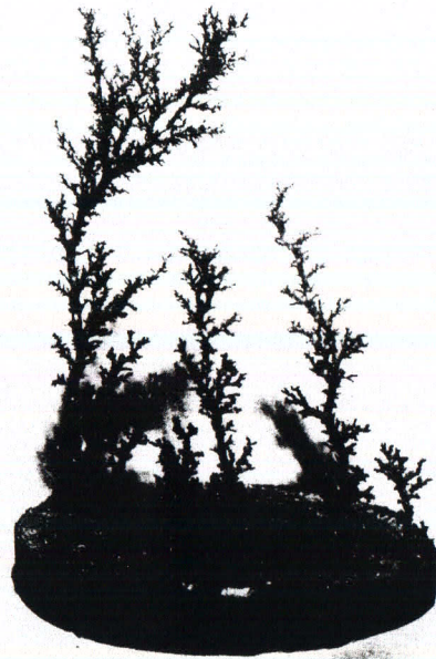
Figure 10.16. Three-dimensional trees obtained at the end of an experiment on chemical dissolution. These structures are made of Wood's metal which was used to fill the channels previously etched by water injected into plaster (Daccord and Lenormand 1987).
