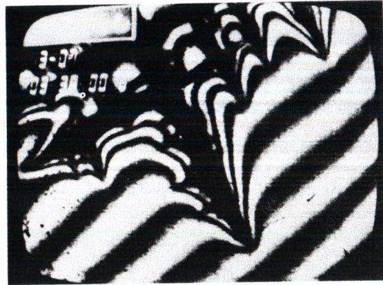
Figure 13.3. Interferogram of the concentration field around a growing \text{NH}_4\text{Cl} dendrite (Raz et al 1989). The stripes, just like equipotential lines, correspond to places with roughly the same concentration.
