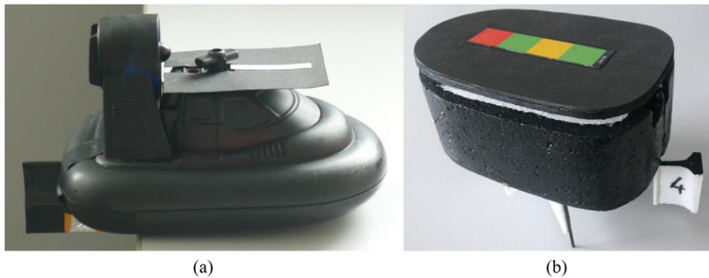
**Figure 2.** The simple robotic units. (a) The commercial boats used in the experiments were modified: superfluous parts removed, rudder fixed, painted black, retroreflective stripe attached; (b) custom-made steerable leader boats with similar properties to the normal boats, but with coloured unique barcode IDs on top.
