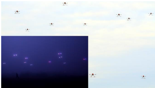
Figure 4. Snapshots of quadcopter flocks of 10 units. Nightlight image: robots are following a target in a grid formation ( r_0 = 6 m, v_0 = 3 m/s). Daylight image: SPP model ( r_0 = 10 m, v_{\text{flock}} = 2 m/s).
